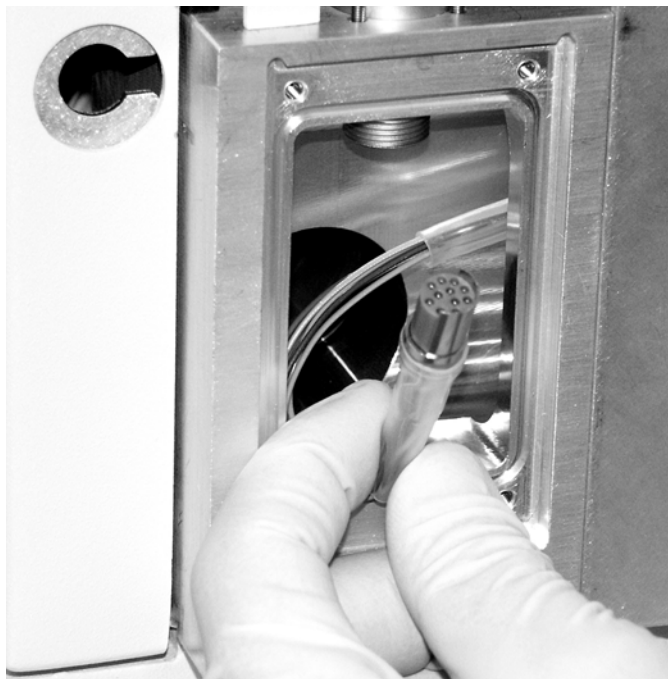
Figure 52. Unplugging the ion source cable harness connector
