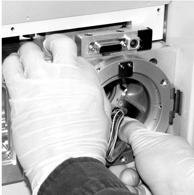
Figure 55. Removing the ion optics cage assembly
